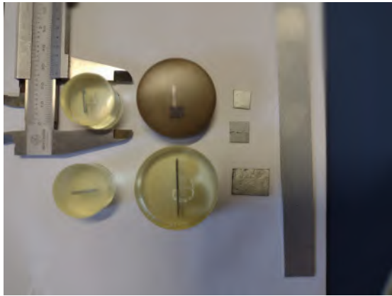
Figure 2: Some steel samples cut and some samples embedded in bakelite.
